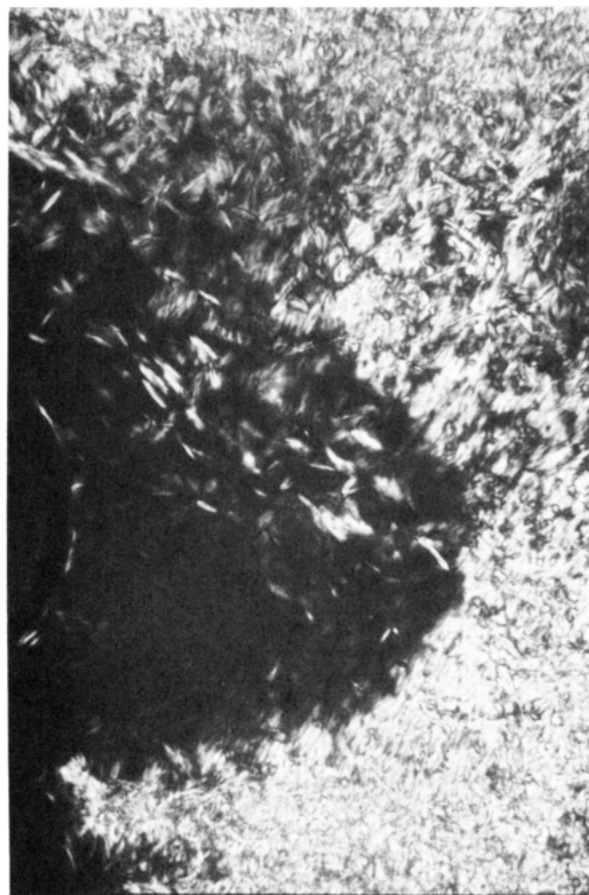
Figure 7. Optical micrograph showing the mesophasic texture of the PD8 polymer at 263 °C on cooling from isotropic melt at 2 °C/min. Cross polars; magnification 1050 \times . (The original has been reduced 40%.)
