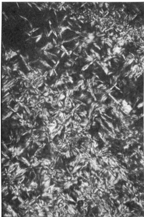
Figure 8. Optical micrograph of the mesophasic texture for the PD10 polymer at 233 °C on cooling from isotropic melt with a rate of 20 °C/min. Crossed polars; magnification 1050 \times . (The original has been reduced 40%.)
